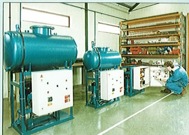
Three JM(UK) sets in production for a soap factory in Indonesia. Because of the damp climate the control panels included special heaters.
